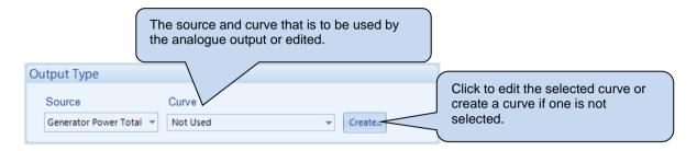
When creating a new sensor curve the measurement quantity and measured parameter are required.
