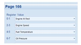
The register address is obtained from the formula: register\_address=page\_number\*256+register\_offset. To read the *Engine Speed* from the above register, the MODBUS master device needs to read the data in two registers and then combine the data from the Most Significant Bit and the Least Significant Bit. MSB address in Decimal = (166 \* 256) + 2 = 42498 LSB address in Decimal = (166 \* 256) + 3 = 42499
